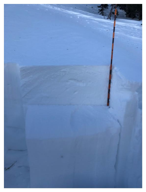
We found unstable stability test scores (ECTP 11) in this pit. And this drift collapsed with an audible "whumph" and cracks 30 feet wide. A buried layer of surface hoar and facets collapsed under a hard slab that formed from strong winds last night. Photo: GNFAC
