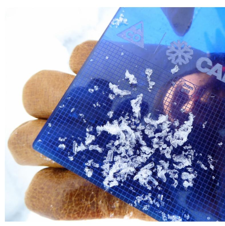
This is a close-up of the angular Depth Hoar grains found near the ground in the mountains south of Big Sky to West Yellowstone. These are weak and cannot support a lot of snow weight. Avalanches will break near the ground on these. Photo: GNFAC
