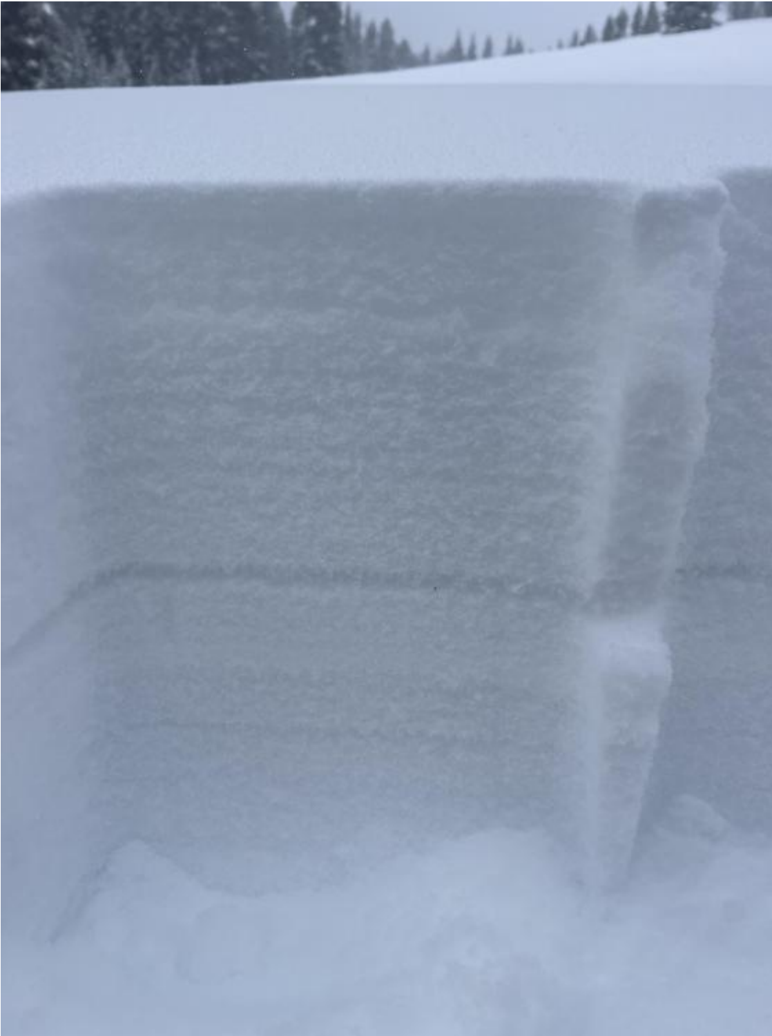
Buried SH below the 2/1 storm. 1-2cm thick layer buried approximately 20cm deep below F precip particles. Photo: M Zia
