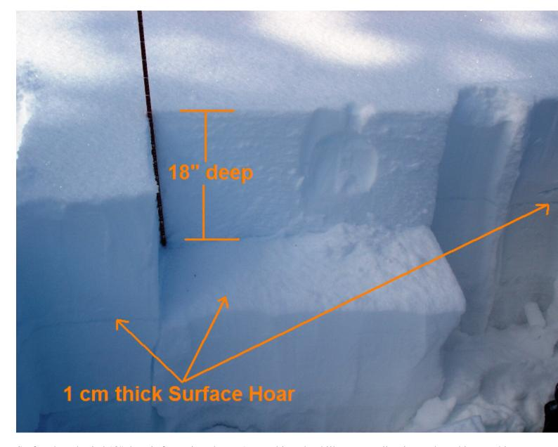
Surface hoar buried 18" deep is fracturing clean. As we skinned uphill we got collapsing and cracking on this layer. Our Extended Column Test propagated with 5 taps (see video). Isolating a column for a compression Test the surface hoar broke before I even tapped it (CTV, Q1). This slope was 20 degrees steep and east facing in the southern Madison Range. Photo by GNFAC
