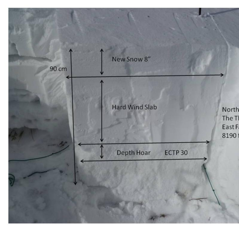
New snow and strong winds produced a thick slab resting over facets. Although it took some force for the ECT to propagate, we did not trust the structure. Photo: GNFAC
