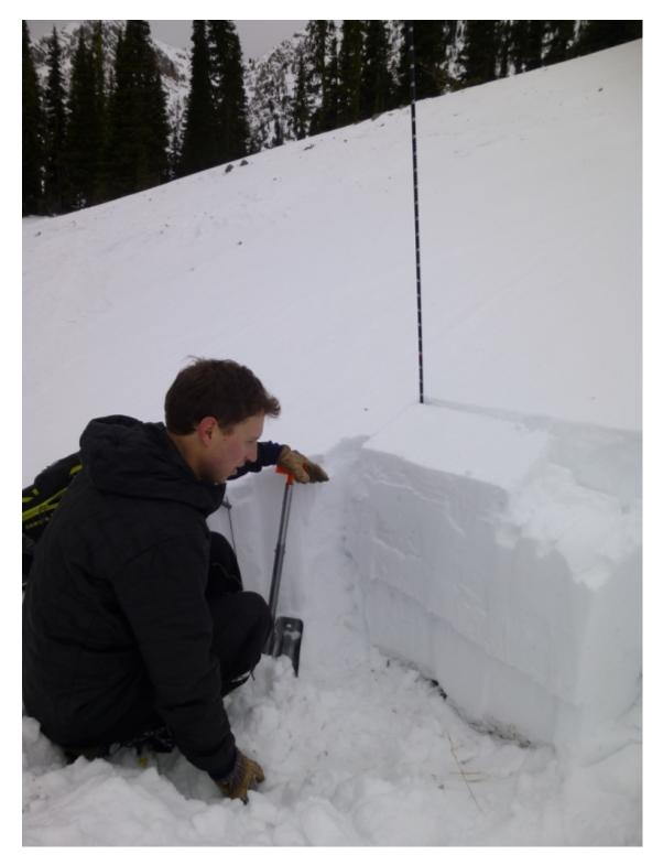
This pit was dug on a wind loaded slope with small facets under the wind slab. It broke clean in our stability tests. Luckily this instibility is not found in most areas, but it's worth searching for. ECTP18. Photo: GNFAC
