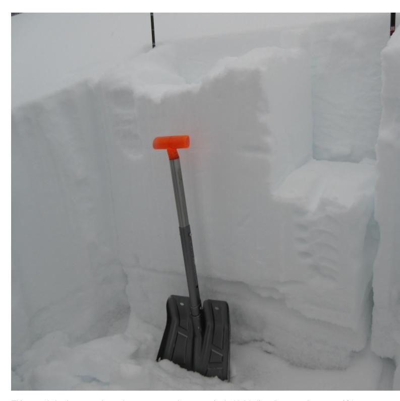
This extended column test shows the poor snowpack structure in the N. Madison Range on January 6, 2016. ECTP 30. Despite difficult initiation, poor structure that has been propagating and causing avalanches for weeks had us sticking to low angle slopes. Photo: GNFAC
