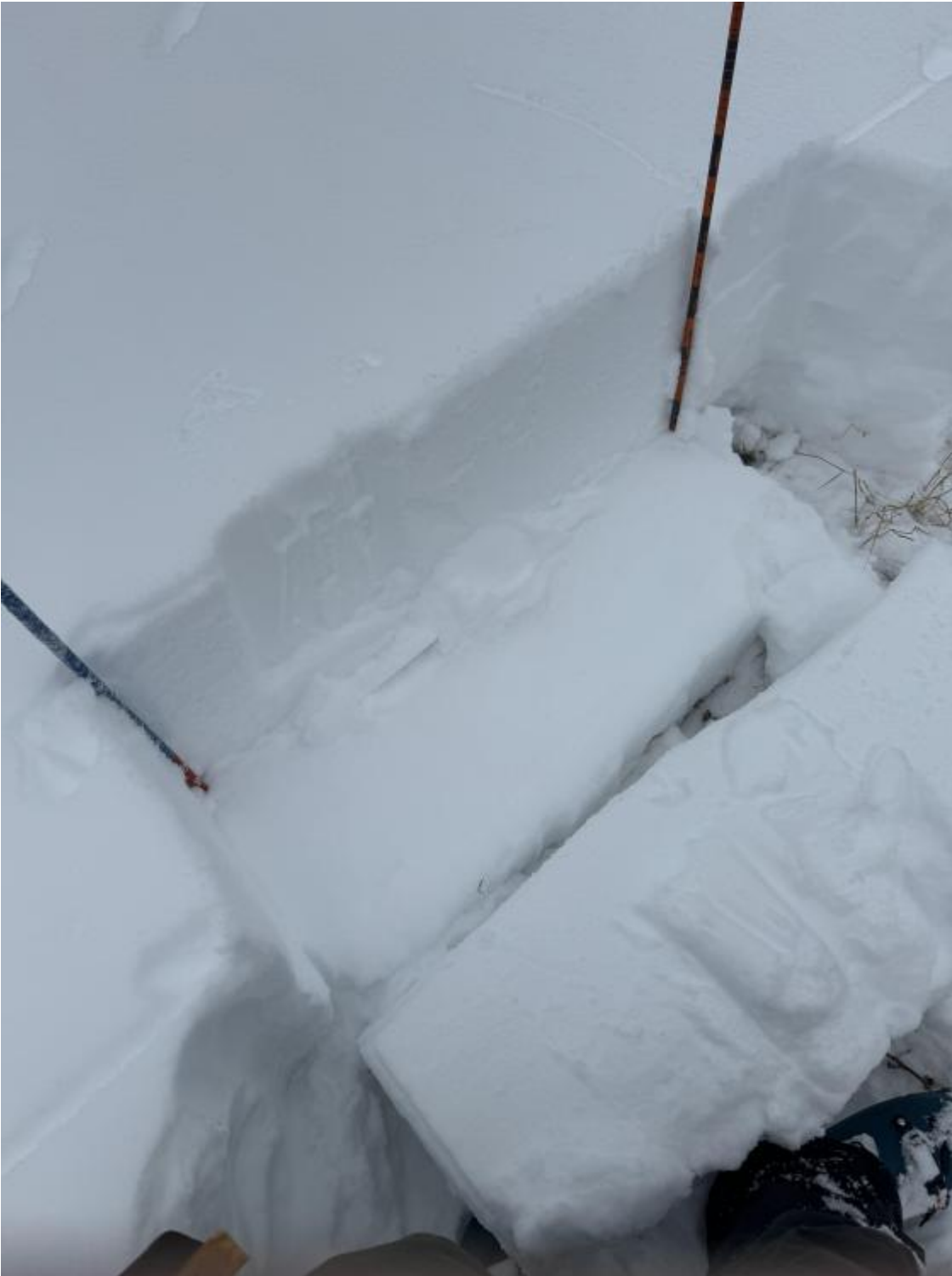
Multiple pits yielded propagation in ECTs for a group in Beehive Basin on Saturday. Photo: E. Stutzman
